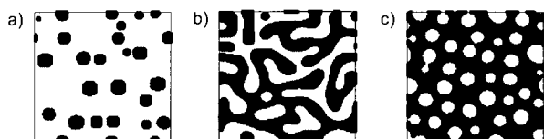
Figure 4. Schematic representation of the growth of the antiferromagnetic (white) and superconducting (black) phases with increasing doping or \delta value (reproduced with permission from ref. [10]).
